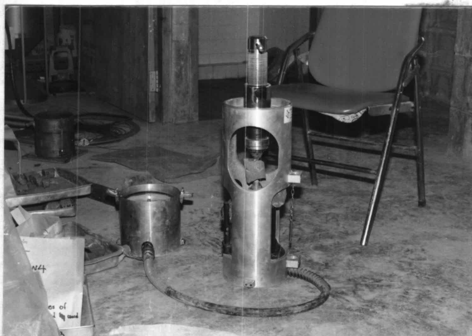
Figure 4.11 The point-load test machine being worked on the pebbly graywacke core specimens.
