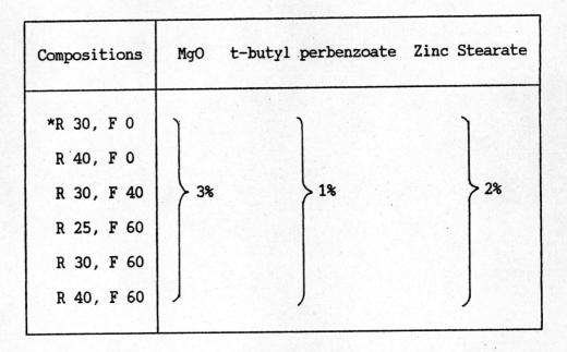
Note \* R 30 : 30% by weight of glass fiber in the resin mix, F0 : 0% or no  $CaCO_3$  in the resin
