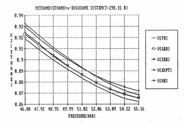
Figure 5.5 Comparisons of experimental and predicted ethane mole fraction by SRK, HK, G&D and PR equations of state(k, =0) as a function of pressure for vapor phase of Methane(1)+Ethane(2)+n-Docosane(3)system.[Data from Jangkamolkulchai, A. and Luke, K.D.(1989).]
