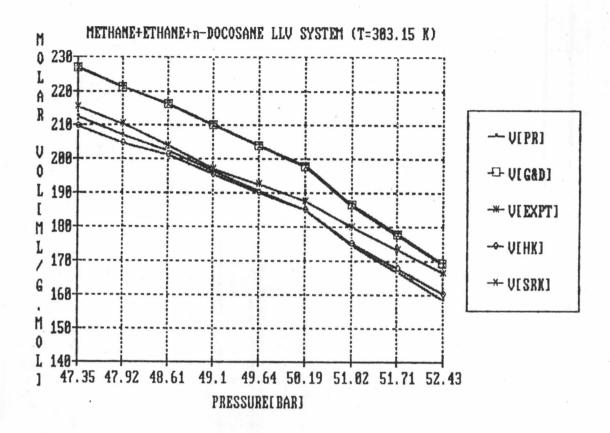
Figure 5.16 Comparisons of experimental and predicted molar volume by SRK, HK, G&D and PR equations of state(k, =0) as a function of pressure for vapor phase of Methane(1)+Ethane(2)+n-Docosane(3)system.
