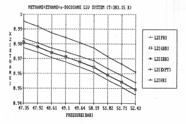
Figure 5.12 Comparisons of experimental and predicted ethane mole fraction by SRK, HK, G&D and PR equations of state( $k_{i,j}=0$ ) as a function of pressure for  $L^{i,j}$  phase of Methane(1) +Ethane(2)+n-Docosane(3)system.
