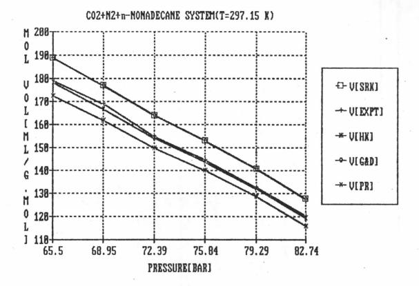
Figure 5.29 Comparisons of experimental and predicted molar volume by SRK, HK, G&D and PR equations of state( $k_{13}=0$ ) as a function of pressure for vapor phase of  $CO_2(1)+N_2(2)+n-Nonadecane(3)$  system.
