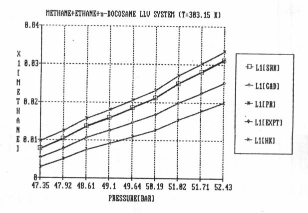
Figure 5.9 Comparisons of experimental and predicted mthane mole fraction by SRK, HK, G&D and PR equations of state(k, =0) as a function of pressure for L' phase of Methane(1) +Ethane(2)+n-Docosane(3)system.
