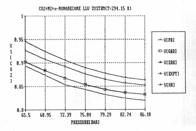
Figure 5.20 Comparisons of experimental and predicted  $CO_2$  mole fraction by SRK,HK,G&D and PR equations of state( $k_{13}$ =0) as a function of pressure for vapor phase of  $CO_2(1)+N_2(2)$ +n-Nonadecane(3)system.
