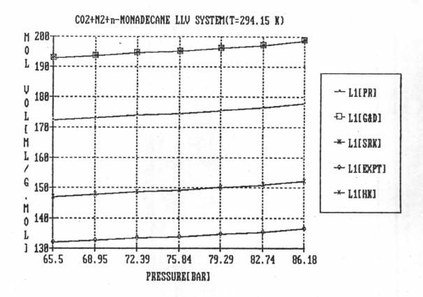
Figure 5.21 Comparisons of experimental and predicted molar volume by SRK, HK, G&D and PR equations of state( $k_{1,3}=0$ ) as a function of pressure for L' phase of  $CO_2(1)+N_2(2)+n-Nonadecane(3)$  system.
