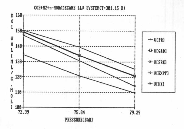
Figure 5.32 Comparisons of experimental and predicted molar volume by SRK, HK, G&D and PR equations of state( $k_{1,1}=0$ ) as a function of pressure for vapor phase of  $CO_{2}(1)+N_{2}(2)+n-Nonadecane(3)$  system.
