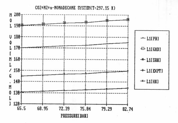
Figure 5.27 Comparisons of experimental and predicted molar volume by SRK, HK, G&D and PR equations of state( $k_{13}=0$ ) as a function of pressure for L phase of  $CO_2(1)+N_2(2)+n-Nonadecane(3)$  system.
