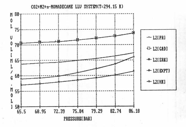
Figure 5.22 Comparisons of experimental and predicted molar volume by SRK, HK, G&D and PR equations of state( $k_{i,j}=0$ ) as a function of pressure for  $L^{11}$  phase of  $CO_2(1)+N_2(2)+n-Nonadecane(3) system.$
