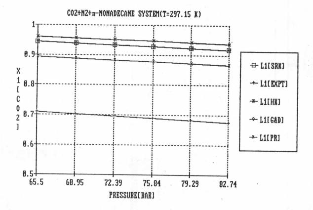
Figure 5.24 Comparisons of experimental and predicted  $CO_2$  mole fraction by SRK, HK, G&D and PR equations of state( $k_{13}=0$ ) as a function of pressure for  $L^1$  phase of  $CO_2(1)+N_2(2)+n-Nonadecane(3)$  system.
