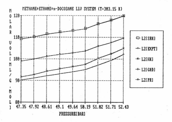
Figure 5.15 Comparisons of experimental and predicted molar volume by SRK, HK, G&D and PR equations of state( $k_{13}=0$ ) as a function of pressure for  $L^{11}$  phase of Methane(1) +Ethane(2)+n-Docosane(3)system.
