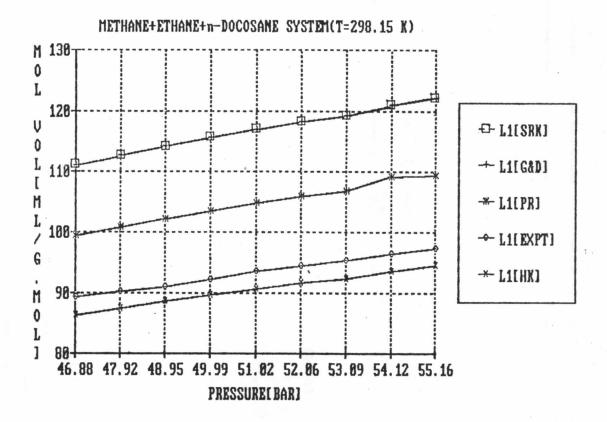
Figure 5.6 Comparisons of experimental and predicted molar volume by SRK, HK, G&D and PR equations of state(k, =0) as a function of pressure for L phase of Methane(1)+Ethane(2)+n-Docosane(3)system.
