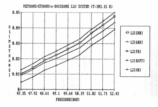
Figure 5.10 Comparisons of experimental and predicted Methane mole fraction by SRK, HK, G&D and PR equations of state(k, =0) as a function of pressure for L' phase of Methane(1)+Ethane (2)+n-Docosane(3)system.
