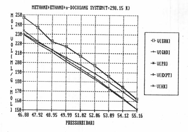
Figure 5.8 Comparisons of experimental and predicted molar volume by SRK, HK, G&D and PR equations of state(k, =0) as a function of pressure for vapor phase of Methane(1)+Ethane(2)+n-Docosane(3)system.
