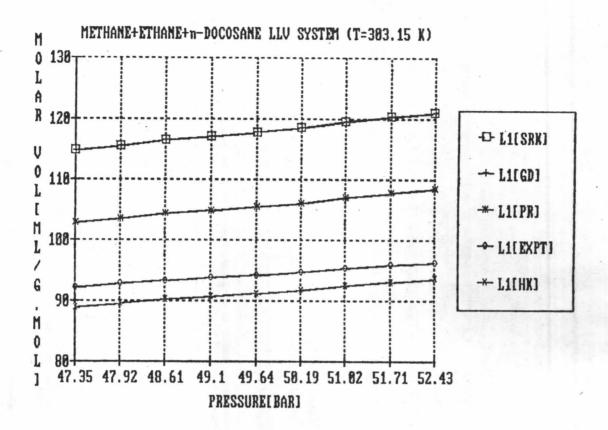
Figure 5.14 Comparisons of experimental and predicted molar volume by SRK, HK, G&D and PR equations of state( $k_{i,j}$ =0) as a function of pressure for L phase of Methane(1)+Ethane(2)+n-Docosane(3)system.
