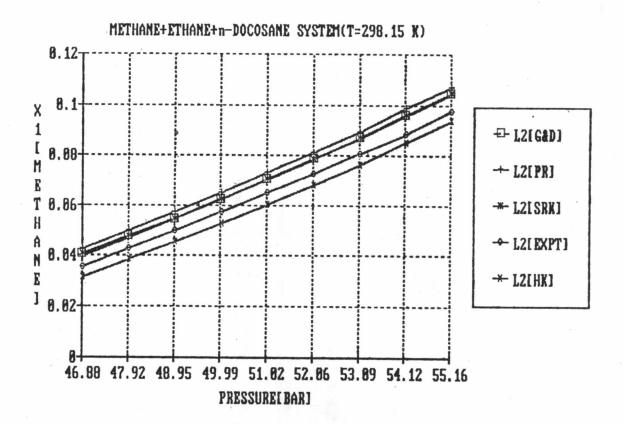
Figure 5.2 Comparisons of experimental and predicted Methane mole fraction by SRK, HK, G&D and PR equations of state( $k_{1,j}=0$ ) as a function of pressure for  $L^{1,j}$  phase of Methane(1)+Ethane (2)+n-Docosane(3)system.
