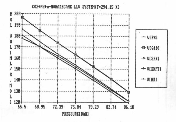
Figure 5.23 Comparisons of experimental and predicted molar volume by SRK, HK, G&D and PR equations of state( $k_{1,1}=0$ ) as a function of pressure for vapor phase of  $CO_2(1)+N_2(2)+n-Nonadecane(3)$  system.
