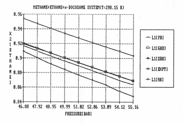
Figure 5.3 Comparisons of experimental and predicted ethane mole fraction by SRK, HK, G&D and PR equations of state( $k_{i,j}=0$ ) as a function of pressure for  $L^{i}$  phase of Methane(1) +Ethane(2)+n-Docosane(3)system.
