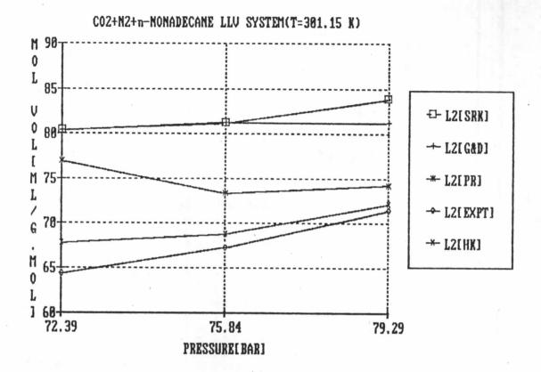
Figure 5.31 Comparisons of experimental and predicted molar volume by SRK, HK, G&D and PR equations of state( $k_{1,1}=0$ ) as a function of pressure for  $L^{11}$  phase of  $CO_2(1)+N_2(2)+n-Nonadecane(3) system.$
