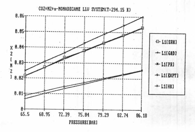
Figure 5.18 Comparisons of experimental and predicted  $N_2$  mole fraction by SRK,HK,G&D and PR equations of state( $k_{1,j}=0$ ) as a function of pressure for  $L^1$  phase of  $CO_2(1)+N_2(2)+n-Nonadecane(3)$ system.
