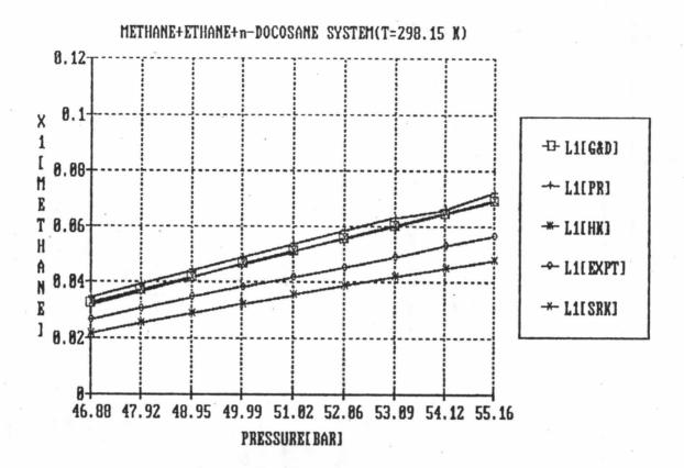
Figure 5.1 Comparisons of experimental and predicted mthane mole fraction by SRK, HK, G&D and PR equations of state( $k_{i,j}=0$ ) as a function of pressure for L phase of Methane(1) +Ethane(2)+n-Docosane(3)system.
