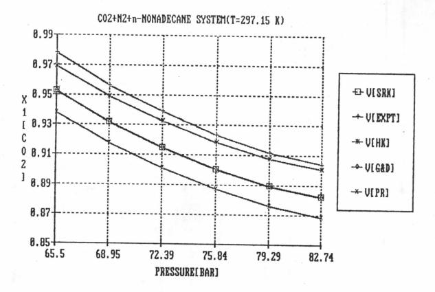
Figure 5.26 Comparisons of experimental and predicted  $CO_2$  mole fraction by SRK,HK,G&D and PR equations of state( $k_{1,1}=0$ ) as a function of pressure for vapor phase of  $CO_2(1)+N_2(2)+n-Nonadecane(3)$  system.
