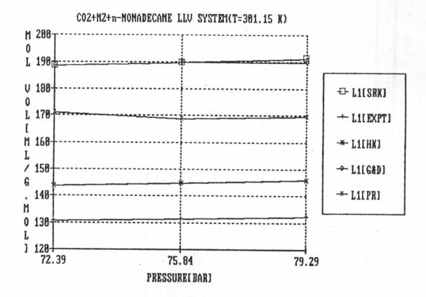
Figure 5.30 Comparisons of experimental and predicted molar volume by SRK,HK,G&D and PR equations of state( $k_{13}=0$ ) as a function of pressure for L phase of  $CO_2(1)+N_2(2)+n-Nonadecane(3)$ system.
