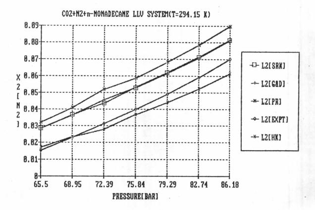
Figure 5.19 Comparisons of experimental and predicted  $N_2$  mole fraction by SRK,HK,G&D and PR equations of state( $k_{13}$ =0) as a function of pressure for  $L^{11}$  phase of  $CO_2(1)+N_2(2)+n-Nonadecane(3)system.$
