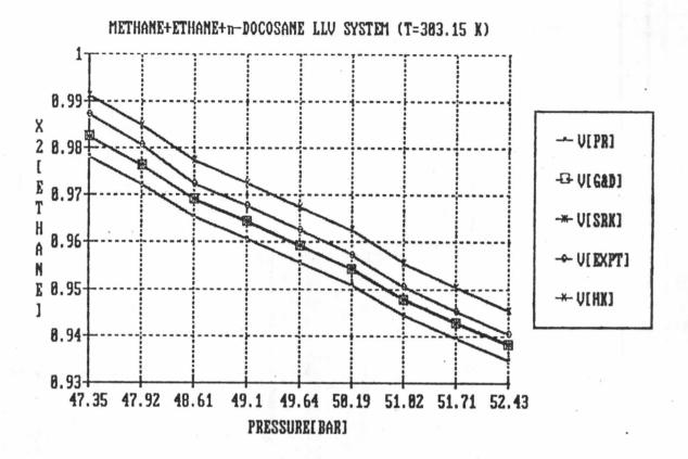
Figure 5.13 Comparisons of experimental and predicted ethane mole fraction by SRK, HK, G&D and PR equations of state(k, =0) as a function of pressure for vapor phase of Methane(1)+Ethane(2)+n-Docosane(3)system.[Data from Jangkamolkulchai, A. and Luke, K.D.(1989).]
