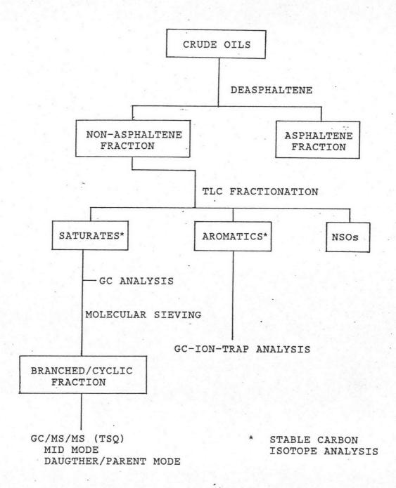
Figure 21. Flow diagram of experimental procedure.
