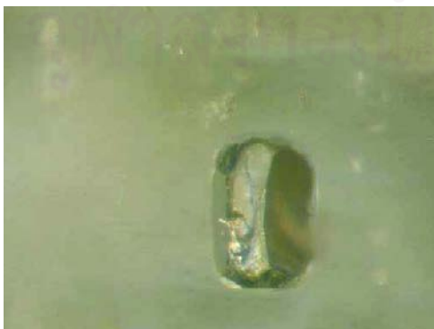
Figure 3.52: Well developed rectangular outlines of high relief negative crystal (MA20, 120x).
