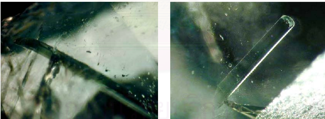
Figure 3.58: elongated prismatic actinolite inclusions in both pictures (high relief); (ZA17, 120x).
