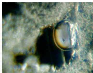
Figure 3.67: Growth tubes containing iron stain and fluids (left); (ZA29, 120x) and primary fluid inclusions (2-phase) showing a high relief gas bubble (right); (ZA29, 140x).
