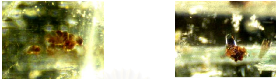
Figure 3.10: Reddish brown to dark brown biotite inclusions in cluster (left) NI10, 70x and book-like appearance (right), d; NI12, 100x.
