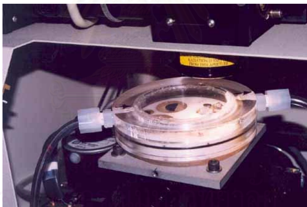
Figure 4.1: Laser ablation Inductively Coupled Plasma Mass Spectrometry Laser Ablation (LA-ICPMS) unit at Macquarie University, Australia used for chemical analysis in this study.
