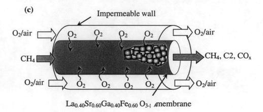
Figure 6.1 Proposed schemes for various OCM reactors (a) FBR (b) PMR and (c) MIECR.
