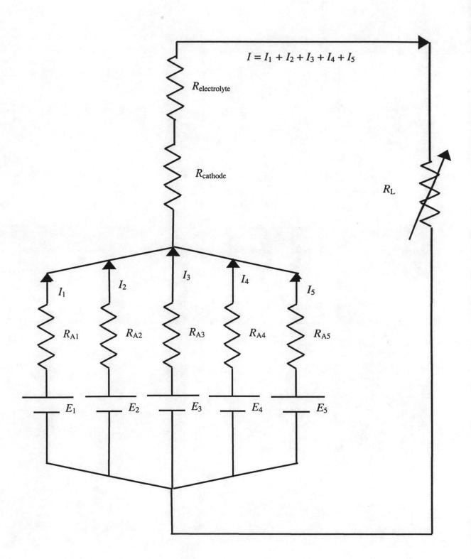
Figure 6.2 Proposed equivalent circuit of SOFC reactor for OCM.
