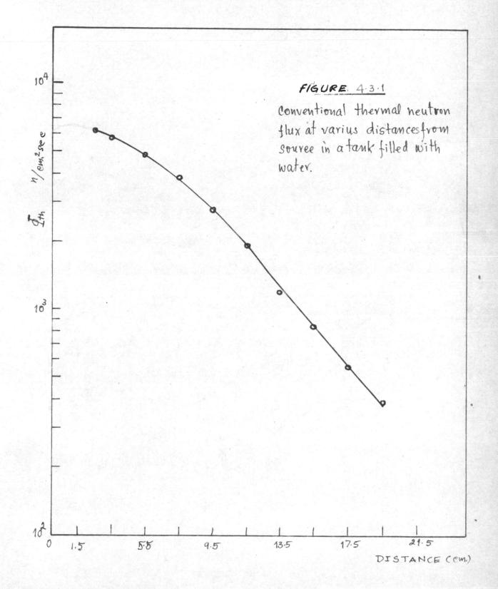
The results of conventional thermal neutron flux at various distance was plotted in Fig. 4.3.1
