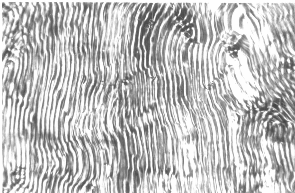
Fig. 13 c) PAA doped with 1 % CP showing cholesteric pitch z_0 \sim 14 \mu\text{m} , at temperature T = 120^\circ\text{C}
