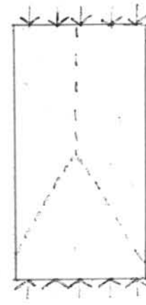
Combining Shear & Splitting Failure
