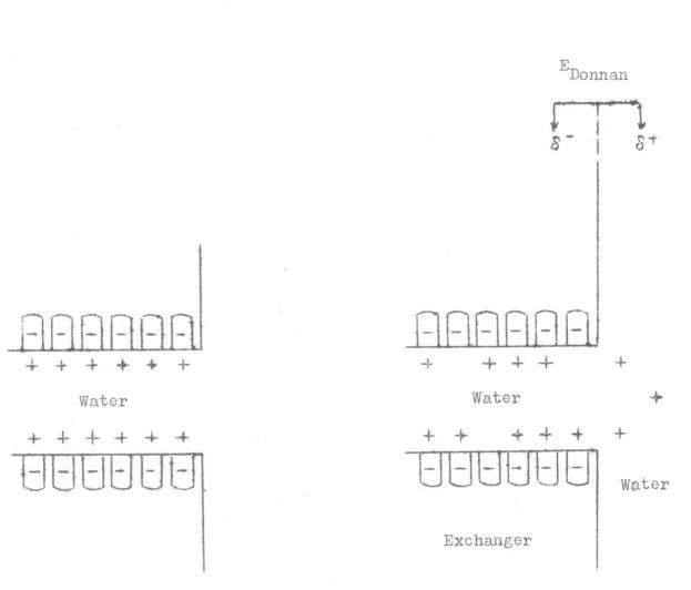
Fig. 2-1 The development of a Donnan potential at an exchanger/solution interface. Left: A hypothetical pore of a cation exchanger before immersion. Right: After immersion in water solvent. matrix sites. The ions of the double layer are never a significant fraction of the exchanger capacity and so electroneutrality within the exchanger phase may be considered to be exactly maintained.
