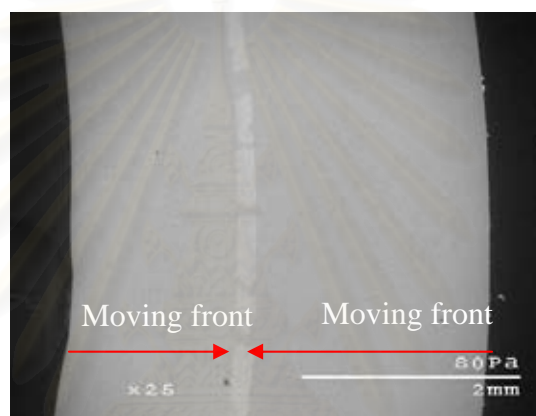
Figure 4.7 Picture of moving-front of TCE penetrating within PVC D after 2 days.
