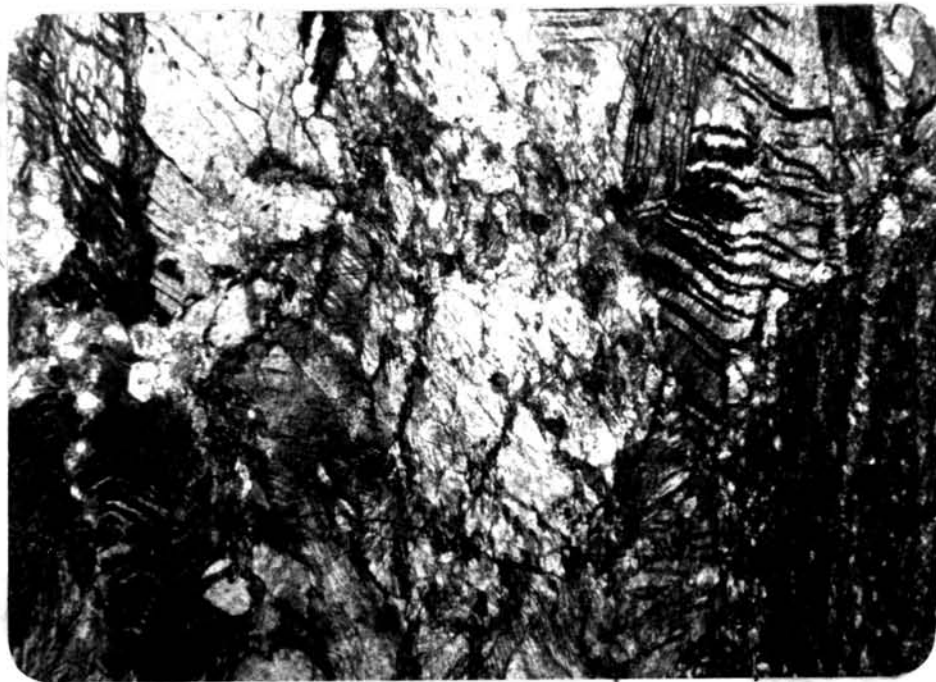
Figure 27 Photomicrograph of light gray limestone showing coarse-grained crystalline calcite and dolomite which exhibit kinking cleavages. (Thin section, 40 x, crossed nicols)
