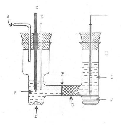
Figure 4. The H cell used in DPP analysis. The labelling letters are A- purified N<sub>2</sub>, B- solution of the sample, C- the DME working electrode, D- Hg, E- carbon rod counter electrode, F- sintered glass disc, G - agar plug, H- the SCE reference electrode, I- saturated KCl and Hg<sub>2</sub>Cl<sub>2</sub> solution, and J- solid KCl, calomel paste and Hg.
