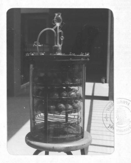
Figure 2 Experimental Glass Jar with Stainless Steel Shelves and Iron Cover.
