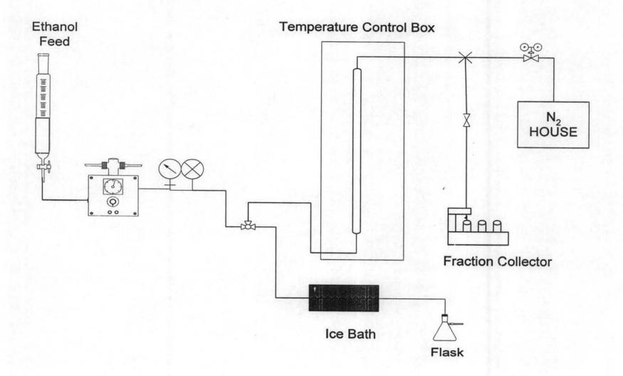
Figure 3.1 Experimental set-up of the dynamic unit.
