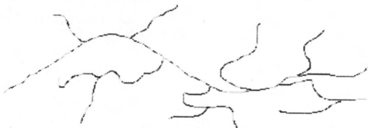
A molecule of branched polyethylene or LDPE
