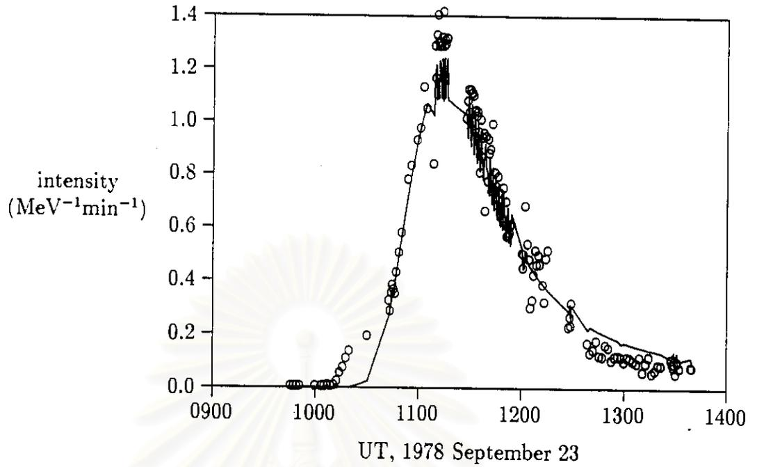
Figure 4.31: Graph of data and simulation of intensity  $\lambda=0.25$  AU for energy 3 Flare September 23.78 (HELIOS I).
