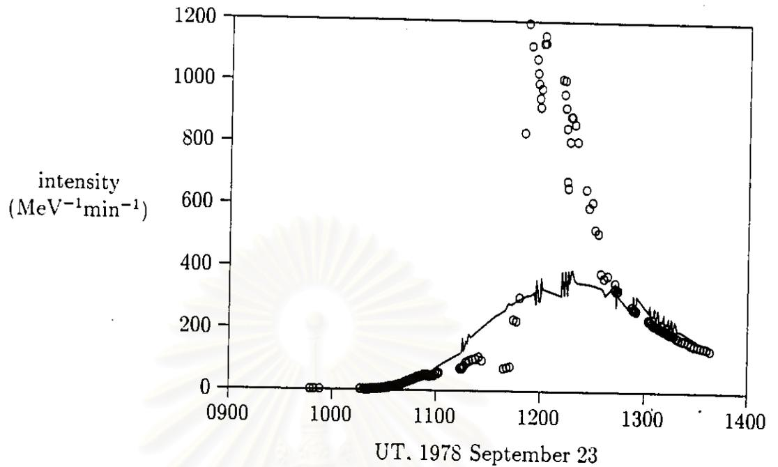
Figure 4.35: Graph of data and simulation of intensity  $\lambda=0.08$  AU for energy 1 Flare September 23.78 (HELIOS II).
