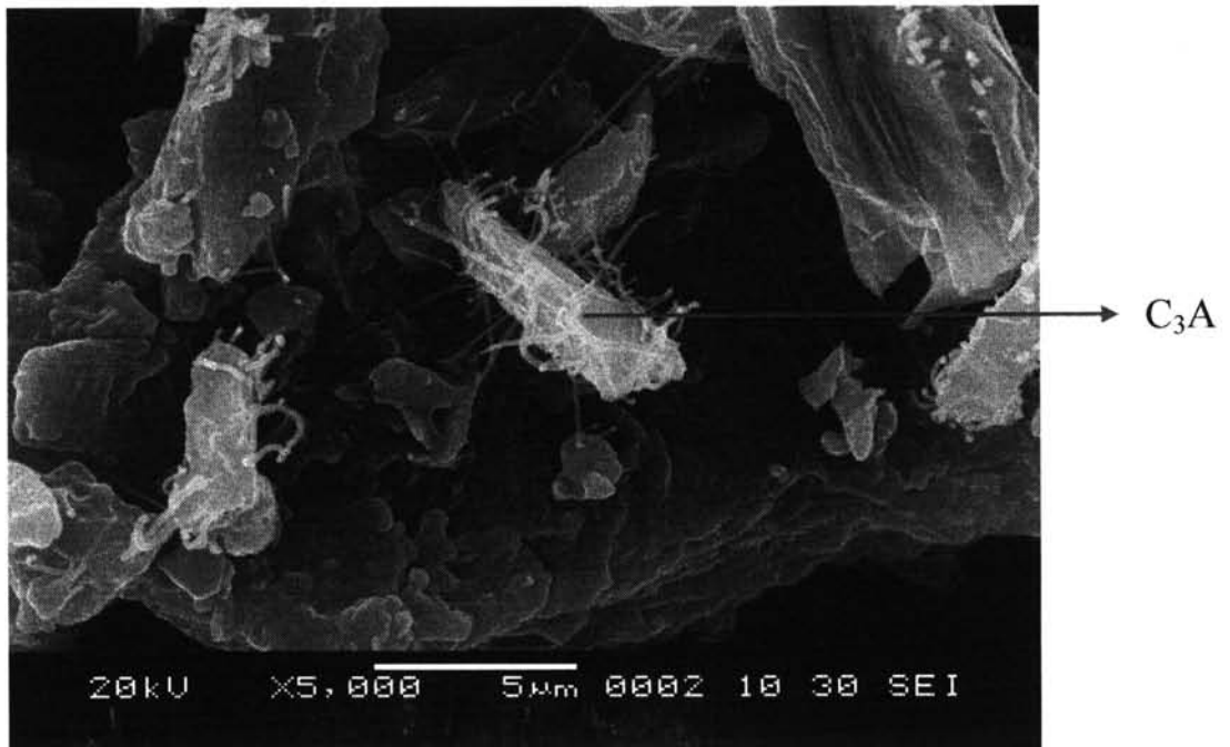
Figure 4.4 Scanning Electron Micrograph 5,000x of the synthetic clinker at 10% replacement
