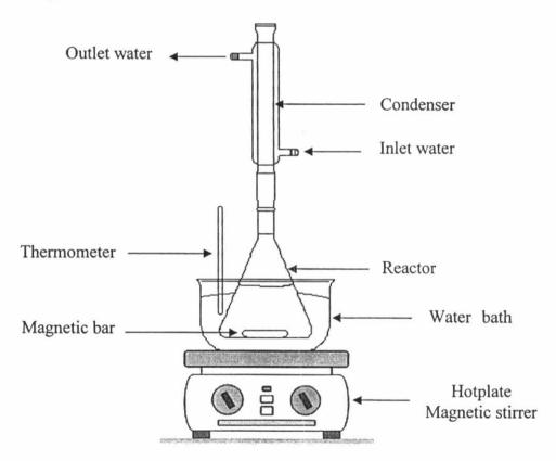
Figure 3.1 Schematic diagram of system
