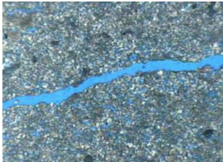
Figure 3.2 Different porosity carbonate rock, showing fractures as secondary porosity
