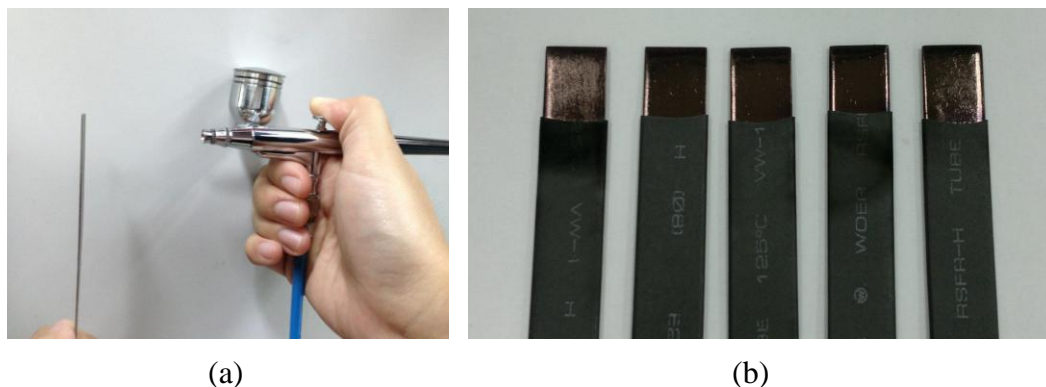
Figure 3.3 (a) Spray gun and (b) Steel coupons coated by spray method
