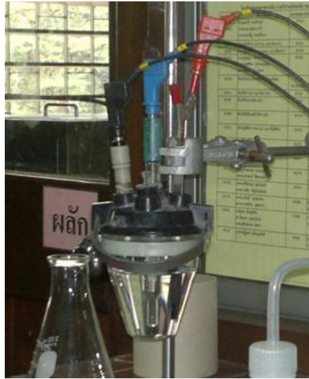
Figure 3.4 The electrochemical Tafel slope analysis apparatus
