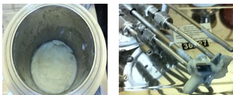
Figure 4.5 The agglomeration of PIP24-CS15A latex in the Parr reactor at high CS15A loading
