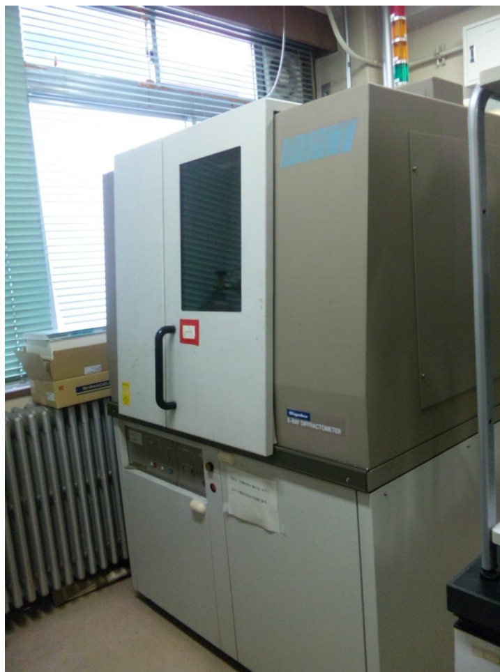
Figure 3.2 XRD diffractometer unit; a Ringaku RINT 2400 X-ray powder diffractometer equipped with \text{CuK}_\alpha radiation
