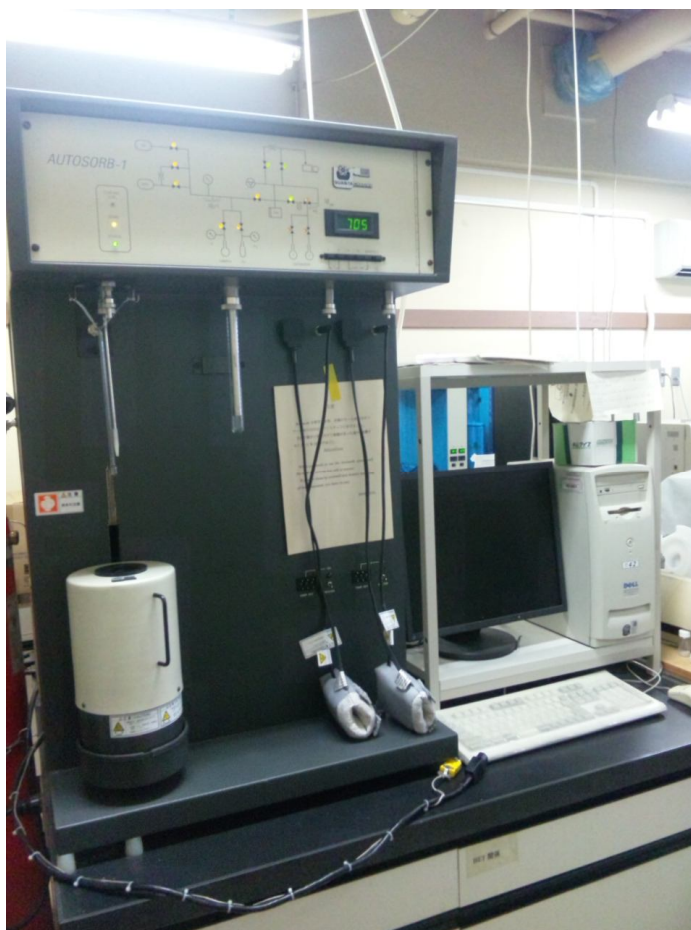
Figure 3.4 An Autosorb-1 (Quantachrome) N 2 adsorption unit
