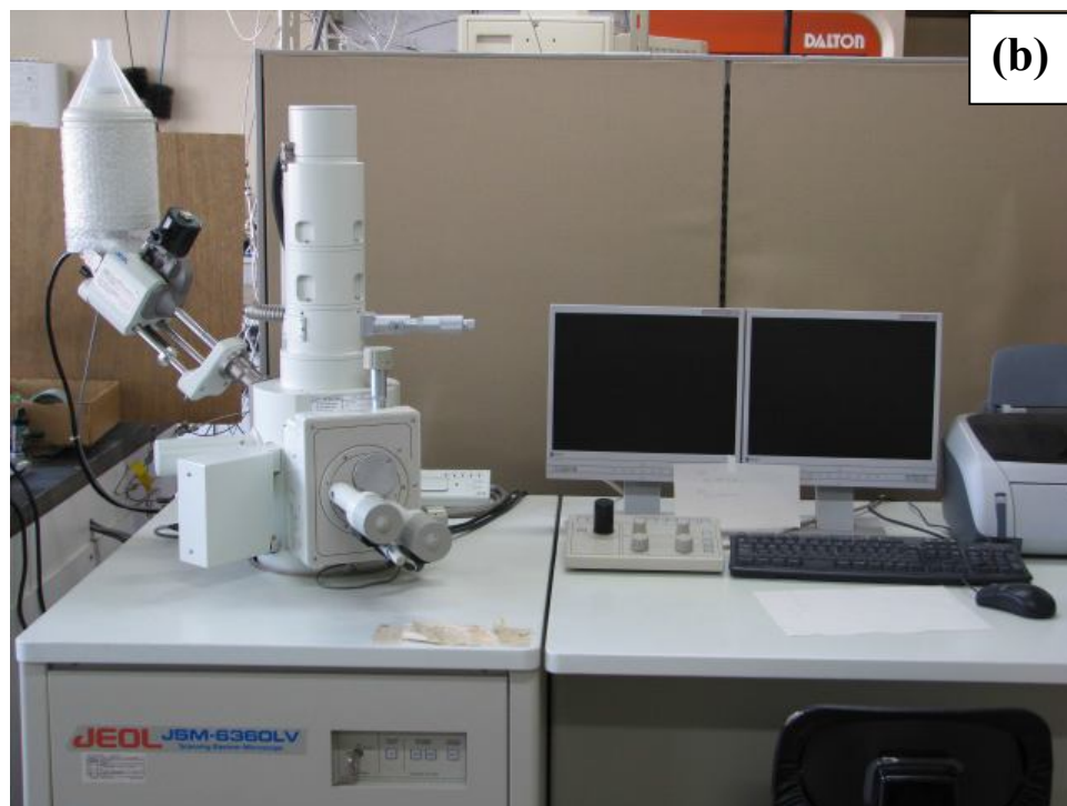
Figure 3.3 Elemental analysis unit; a) an EDX, SHIMADZU Rayny EDX-700, b) an SEM (JEOL JSM-6360LV) equipped with an EDS analysis (EDS, JED-2300)
