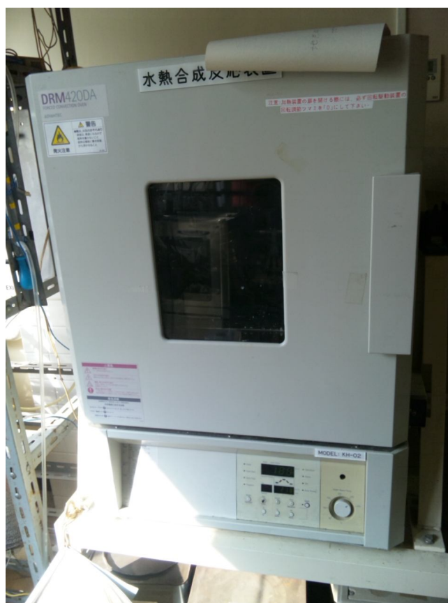
Figure 3.1 Hydrothermal unit apparatus
