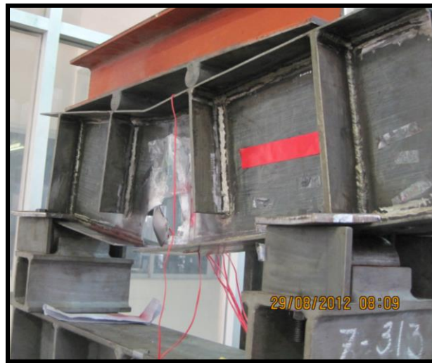
A. Failure of specimen S3-3.
