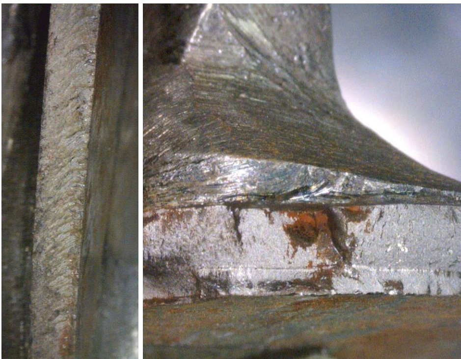
C. Crack surface in propagation and at web-toe.
