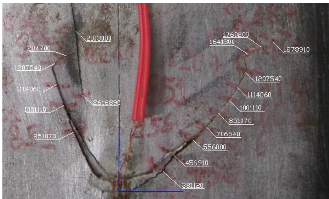
Fatigue crack growth of specimen 2.
