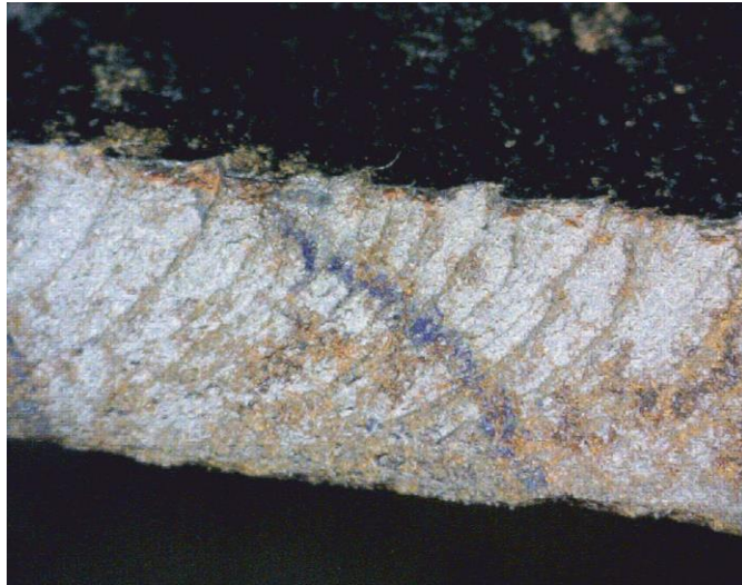
C. Crack surface in propagation.
