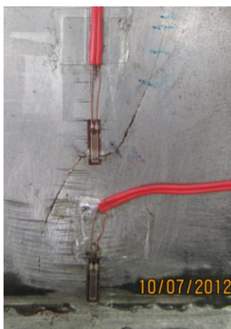
B. Crack before and after failure.
