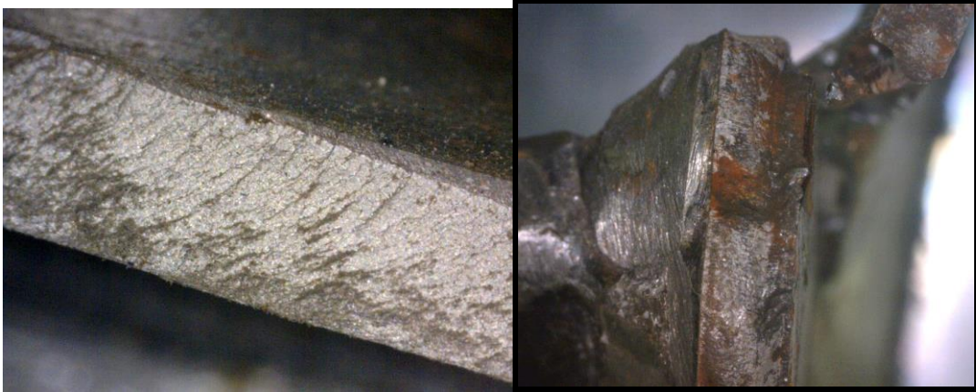
C. Crack surface during growing and at the beginning (weld-toe).
