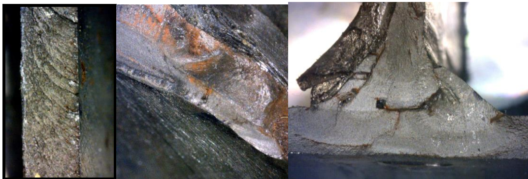
C. Crack surface in propagation, at web-toe and bottom flange.
