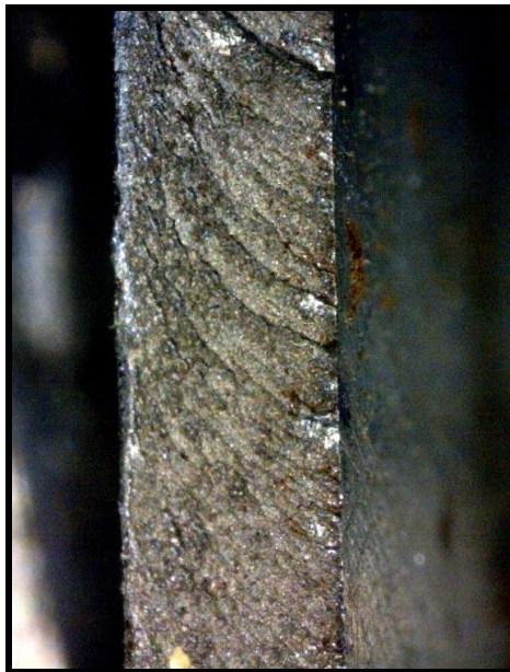
B. First Crack propagation
