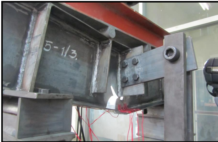
A. Failure of specimen S3-1.
