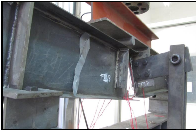
A. Failure of specimen S1-3.
