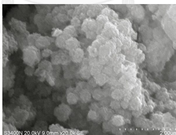
Figure 5. 8 SEM photograph of the zeolite sample synthesized from CFA at large scale
