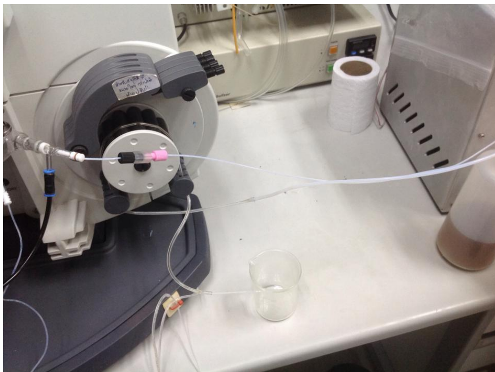
Figure A1-2 The automatic on-line internal standard addition system: the mixture introduction line to ICP-OES and the line for solution loading to sample loop in top view.
