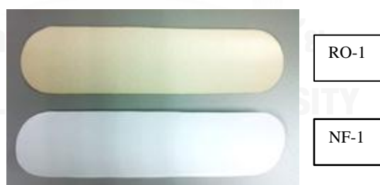
Figure 3.4 RO-1 and NF-1 membranes
