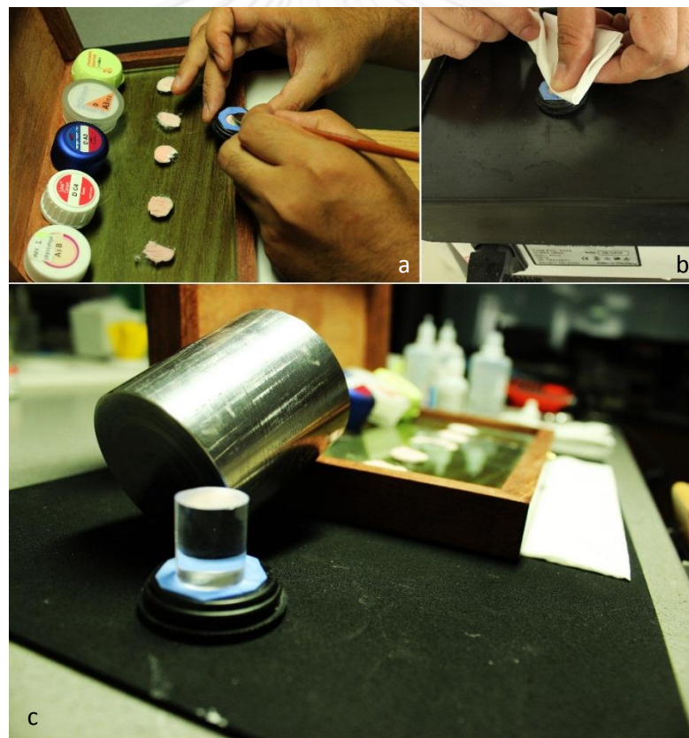
Figure 12. (a) The core was veneered with each veneering porcelain using powder/liquid layering technique. (b) The veneer-core was gently vibrated and blotted dry to remove excess liquid. (c) A 5 kg weight pendulum loaded on the veneering porcelain.
