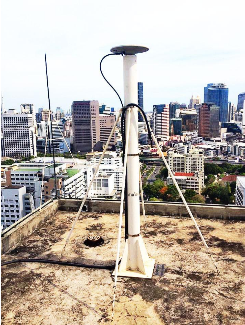
Figure 3.2 Show GPS base CUSV station at Faculty of Engineering, Chulalongkorn University.
