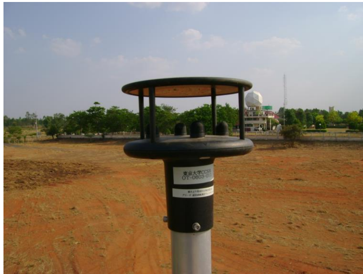
Figure 3.12 Ultrasonic Anemometer at Phimai station.
