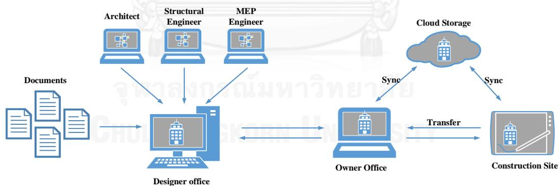
Figure 4.4 System architecture of BIM-based construction project monitoring system
