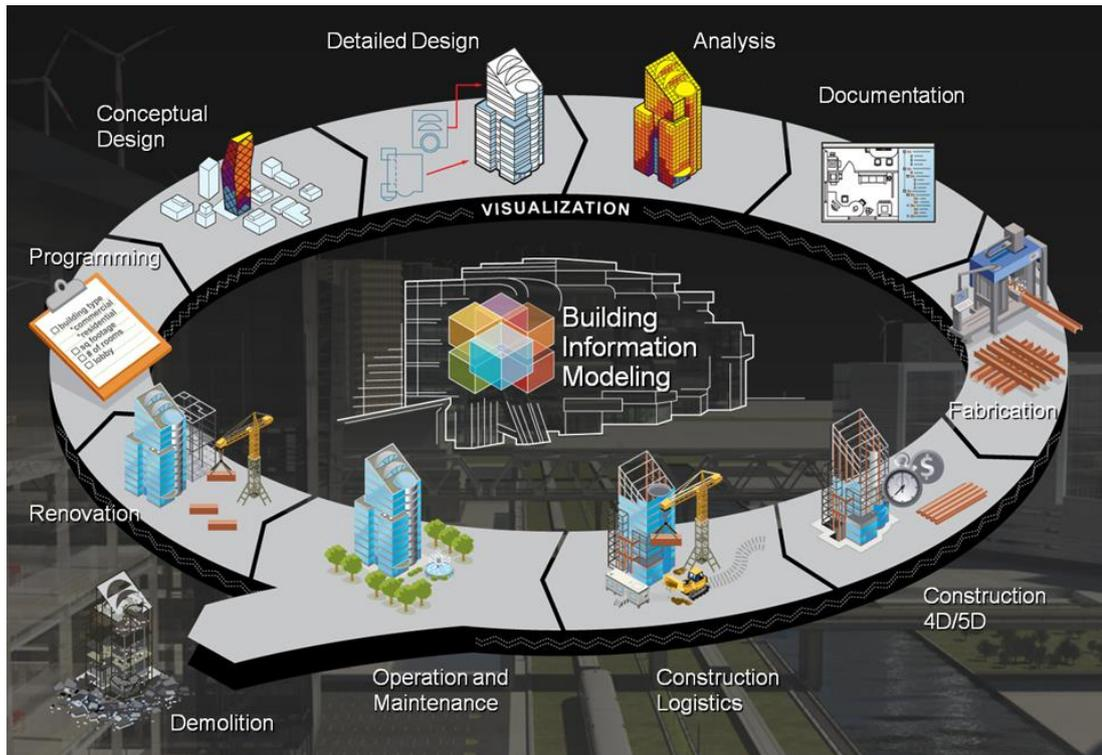
Figure 2.2 BIM-Building life cycle (Source: <http://www.arquibim.es>)
