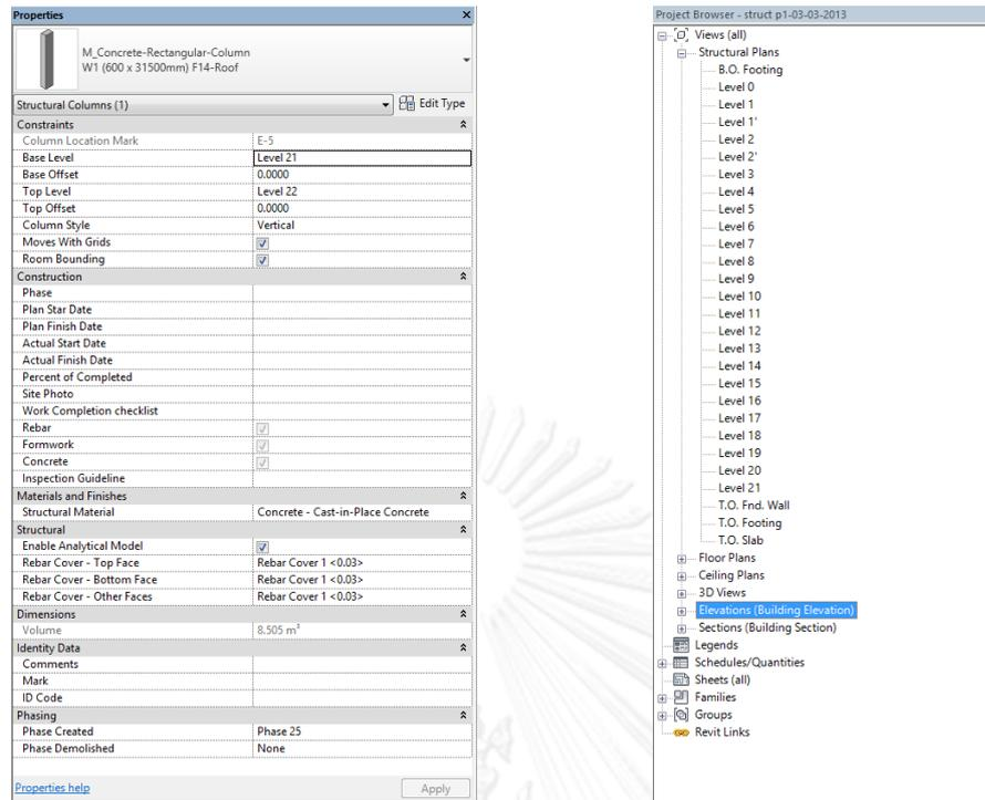
Figure 5.9 Parametric information on BIM-design model
