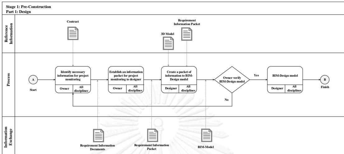
Figure 4.9 Workflow of the BIM-design part
