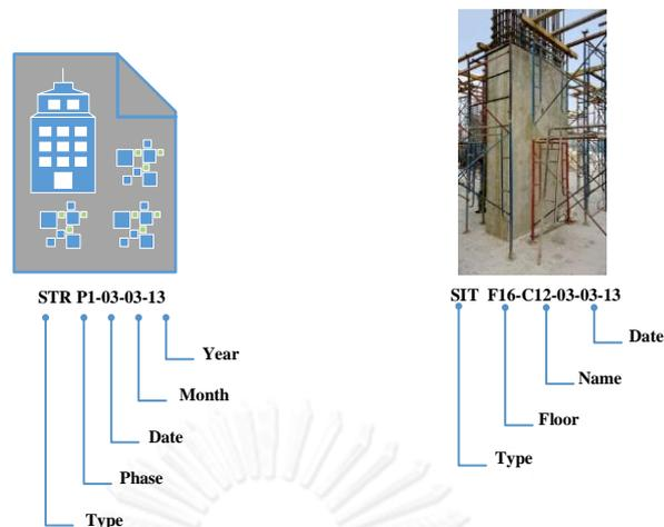
Figure 4.16 File name of BIM-record model for a column
