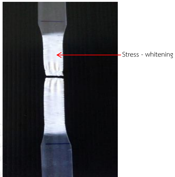
Figure 4.4 The photograph of deformed specimens after tensile testing of PLA/NR film
