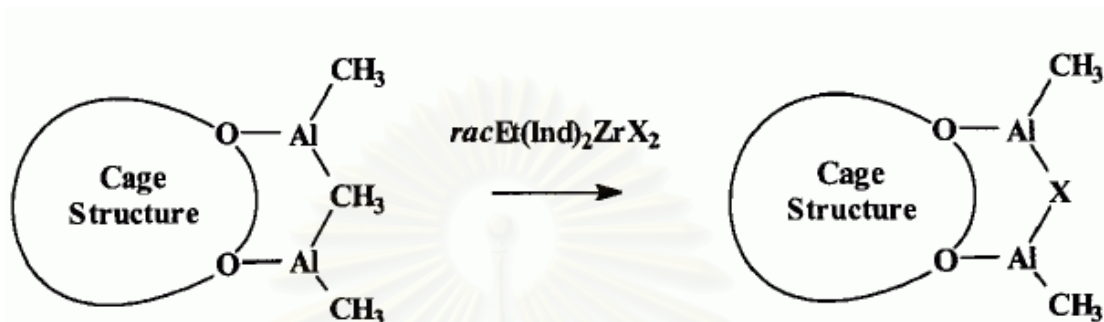
Figure 2.7 Representation of MAO showing the substitution of one bridging methyl group by X ligand extracted from \text{racEt(Ind)}_2\text{ZrCl}_2 ( \text{X} = \text{Cl}, \text{NMe}_2, \text{CH}_2\text{Ph} ) [34].
