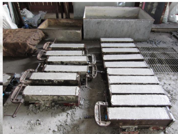
(b) Casting concrete prism
