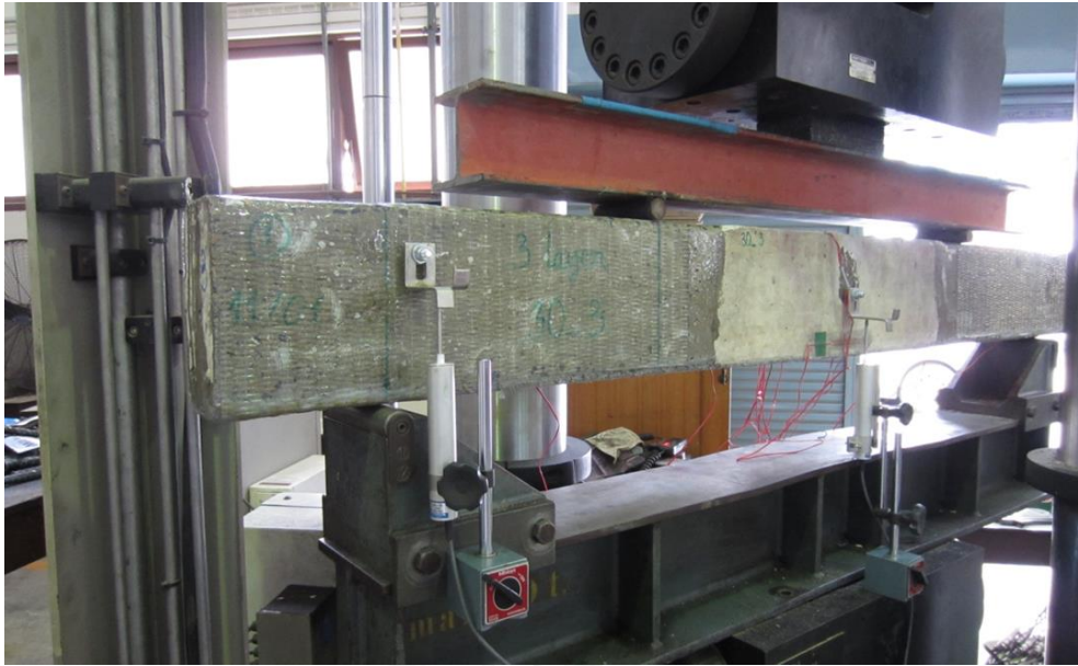
Figure 3. 17 Test setup of bending test
