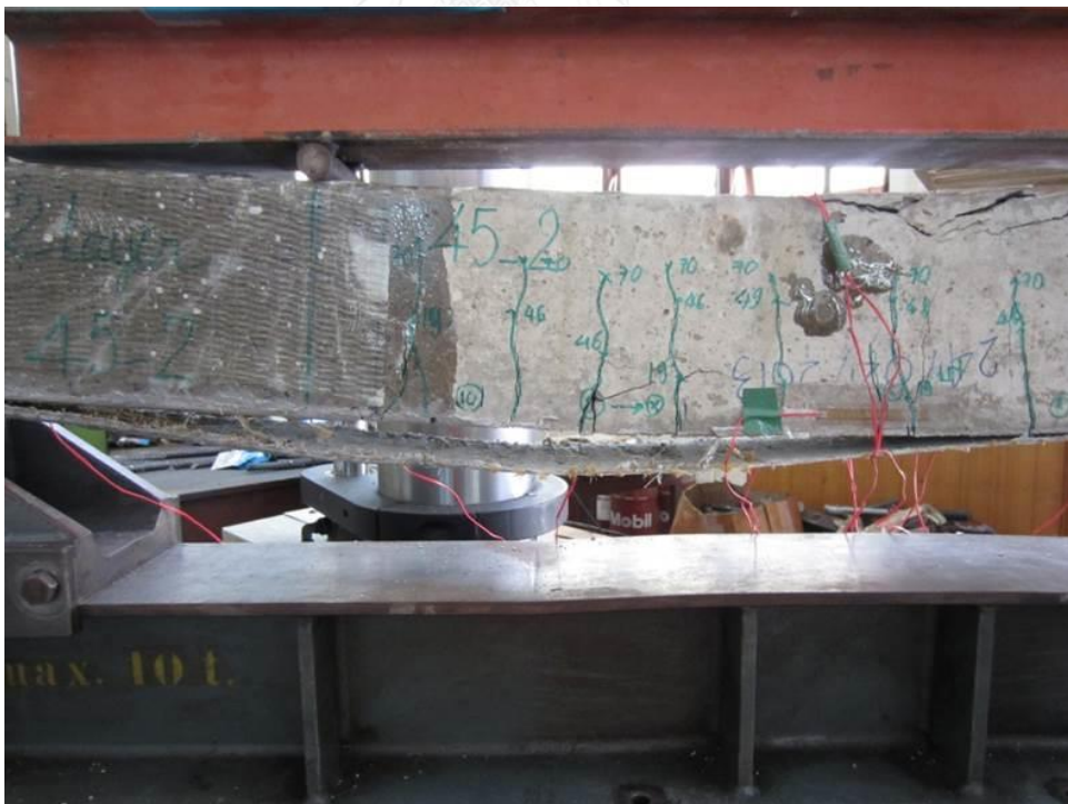
Figure 5. 2 Flexural failure of controlled beam
