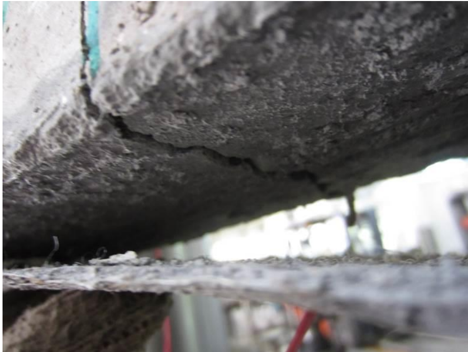
Figure 5. 6 The interface between PBO-FRCM and concrete after debonding
