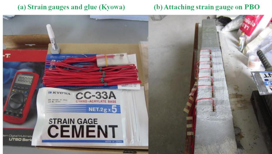
Figure 3. 8 Tested specimen for bond stress-slip test
