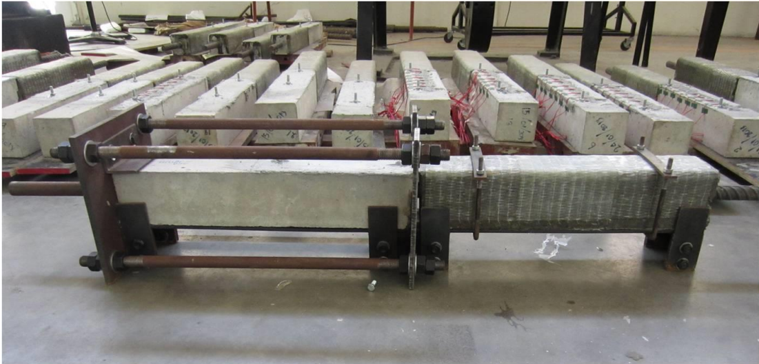
Figure 3.6 Tested specimen in rigid frame
