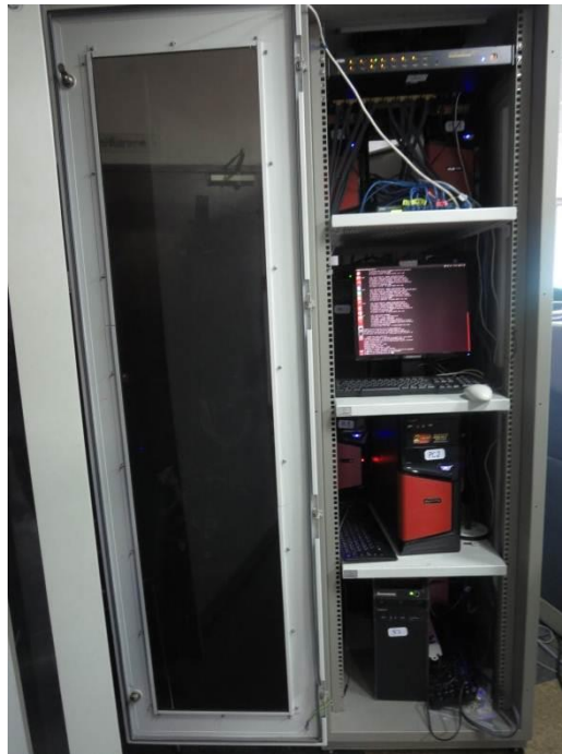
Figure 3. 10: PC-based OpenFlow testbed
