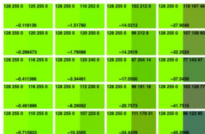
Figure 2.6 An example of calculated \Delta E^* for different shades of green paint (Monovector, 2011)
