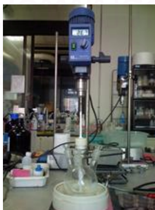
Figure 3.1 Apparatus for ETS-10 synthesis.
