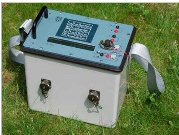
Figure 3.9. SYSCAL R1 Plus Switch 24 - 48 or 72 electrodes spacing between electrodes (std) : 5m ( using to 2-D resistivity survey in study area)
