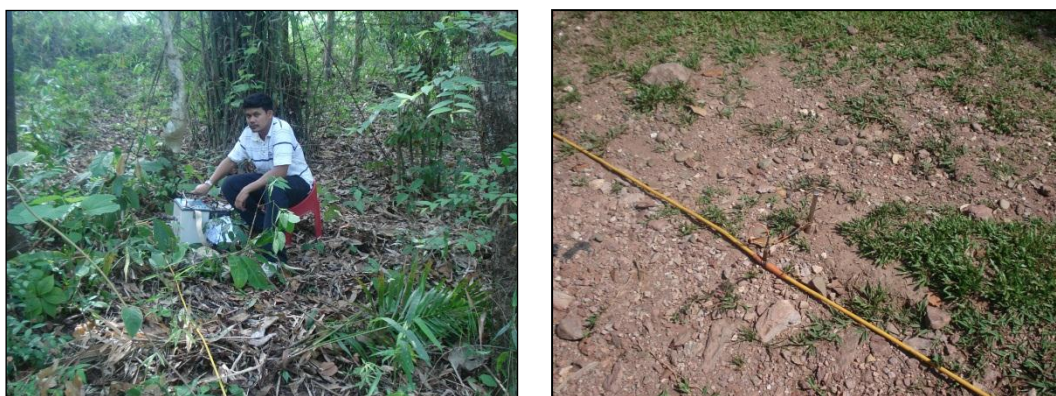
Figure 3.6. 2-D resistivity survey in study area using 48 electrodes (SYSCAL switch multi- electrode equipment )
