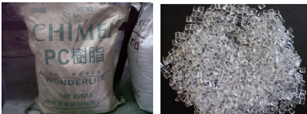
Figure 2.2: Appearance of polycarbonate pellets grade WONDERLITE® PC-110. (Chi Mei Corporation)
