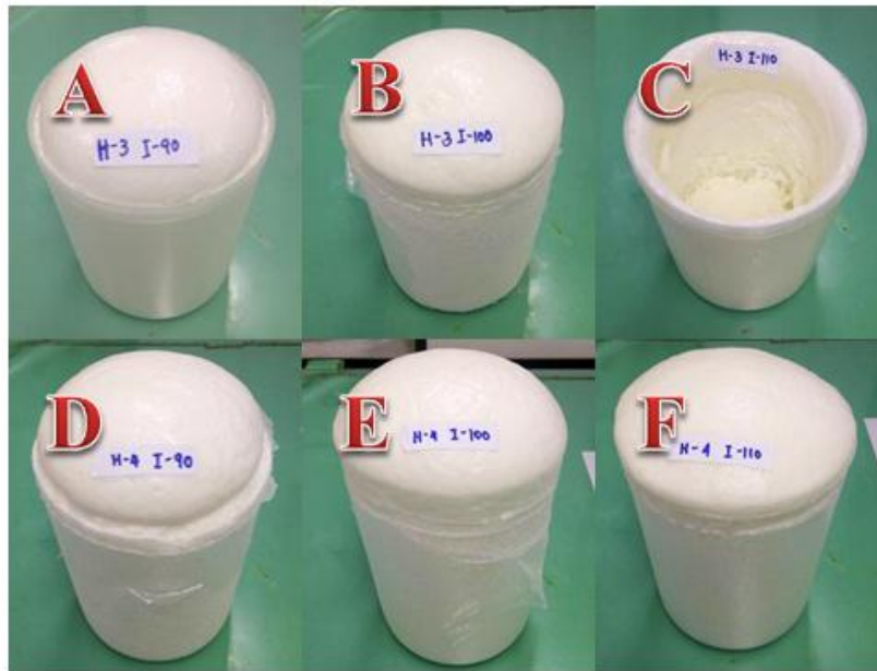
Figure 4.9 FPUR foam appearances prepared from the formulation contained 4.0% water content; (a), (b) and (c) 2.0 pbw cell opening amount at the NCO indexes of 90, 100 and 110, respectively; (d), (e) and (f) 1.5 pbw cell opening amount at the NCO indexes of 90, 100 and 110, respectively
