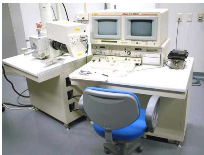
Figure 4.10 Scanning electron microscope (SEM, JEOL: JSM-5410LV, Japan)
