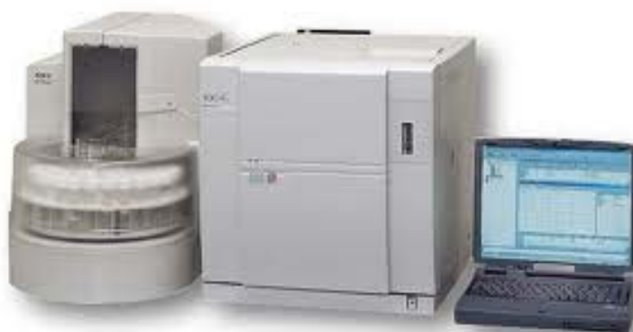
Figure 4.8 Total organic carbon (TOC) analyzer (Shimadzu TOC-V CHP)
