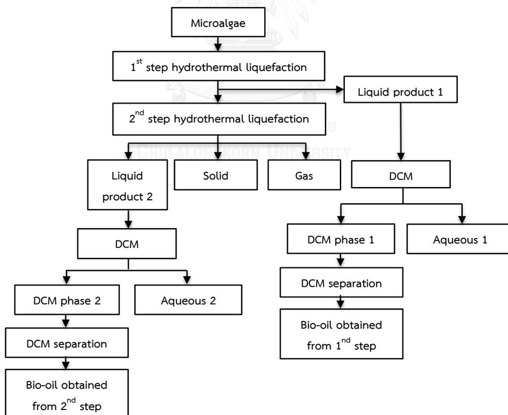
Figure 3.3 Schematic of THTL.
