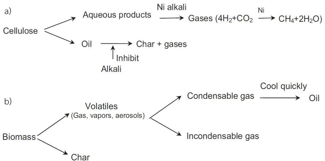
**Figure 2.5** Reaction pathway for the biomass a) hydrothermal liquefaction of cellulose and b) flash pyrolysis process of biomass (Xiu et al., 2012).
