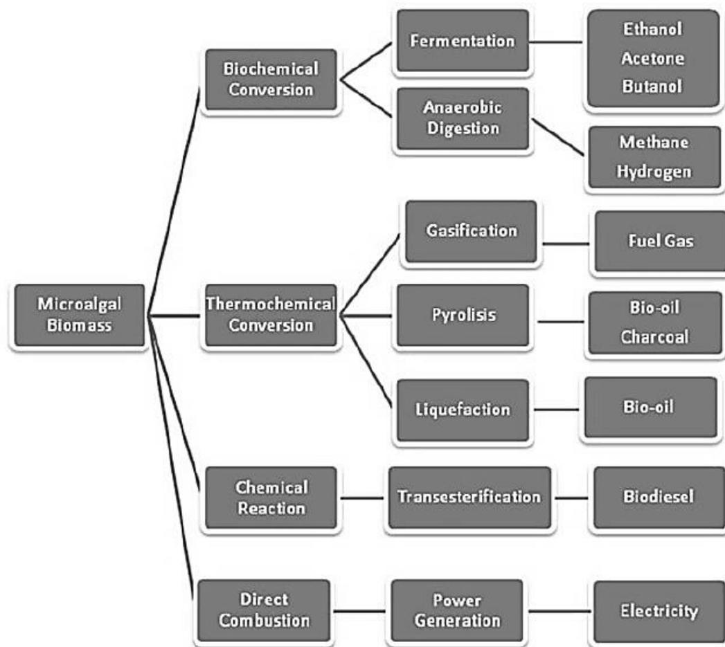
**Figure 2.4** Energy production by microalgae biomass conversion using biochemical, thermochemical, chemical and direct combustion process (Gouveia, 2011).
