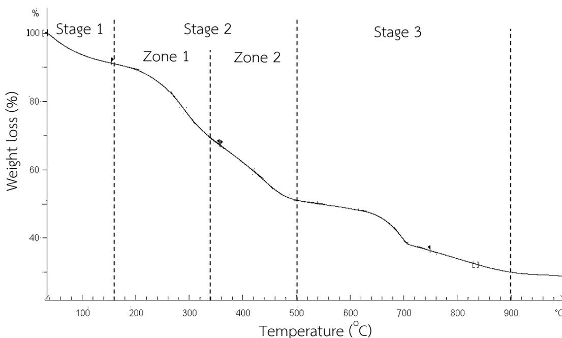
**Figure 4.1** Thermal degradation behavior of microalgae under nitrogen gas (N<sub>2</sub>) (Heating rate of 10 °C/min).
