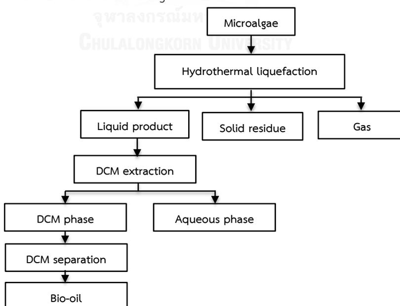
Figure 3.2 Schematic of SHTL.
