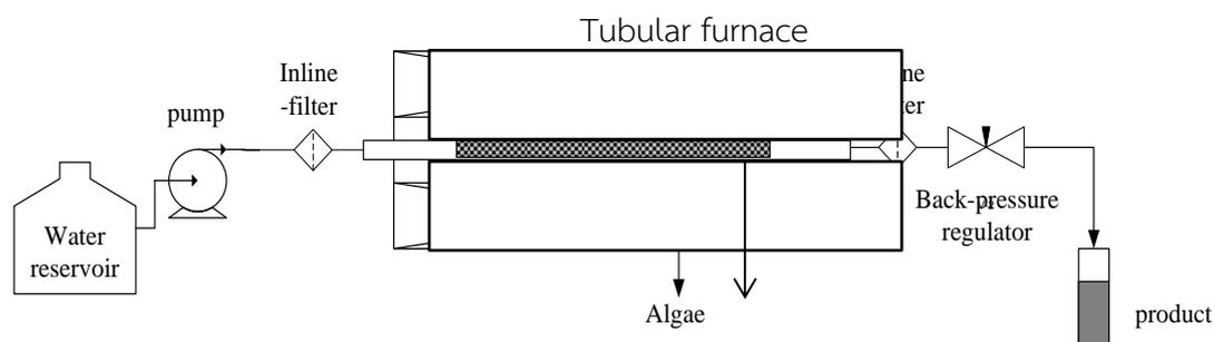
**Figure 3.1** Schematic diagram of hydrothermal liquefaction process.
