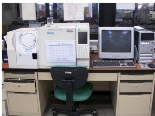
**Figure 3.6** Gas chromatography - mass spectrometry, GC/MS (Shimadzu, GC-2010).
