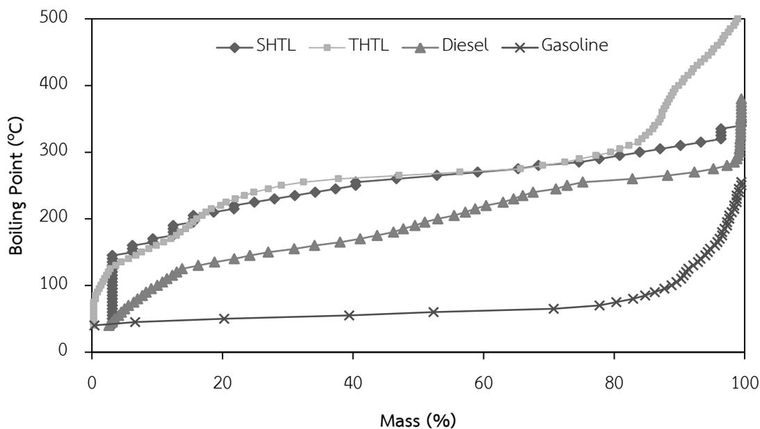
**Figure 4.4** GC-SIMDIS chromatograms of Diesel, Gasoline, Bio-oil obtained from SHTL and the second step of THTL. The SHTL operated at 320 °C under the water pressure of 20 MPa and the water flow rate of 0.50 mL/min. The THTL operated at 200 °C for 1<sup>st</sup> step and 320 °C for the 2<sup>nd</sup> step under the water pressure of 20 MPa and the water flow rate of 0.50 mL/min. Commercial diesel (HSD 0.05%S) and gasoline (UGR 95 RON) were purchased from PTT public company limited.
