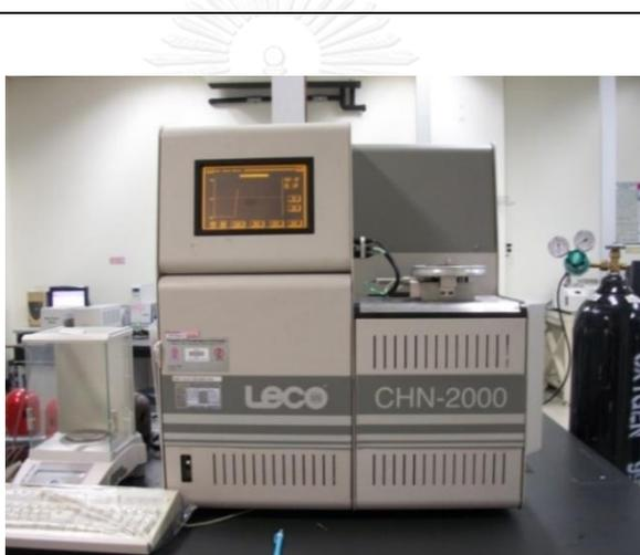
**Figure 3.4** CHN Analyzer (CHN-2000, LECO Instrument (Thailand) Ltd.).
