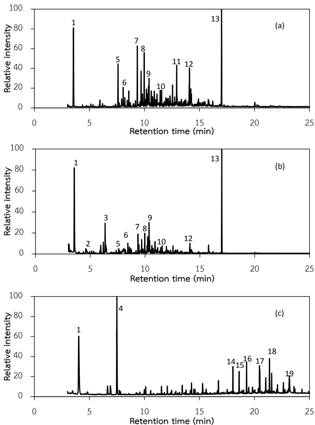
**Figure 4.2** GC/MS chromatograms of bio-oils obtained from (a) SHTL (8.7 wt% of nitrogen content), (b) THTL (4.8 wt% of nitrogen content) and (c) THTL with 10 wt% Na<sub>2</sub>CO<sub>3</sub> (3.7 wt% of nitrogen content).
