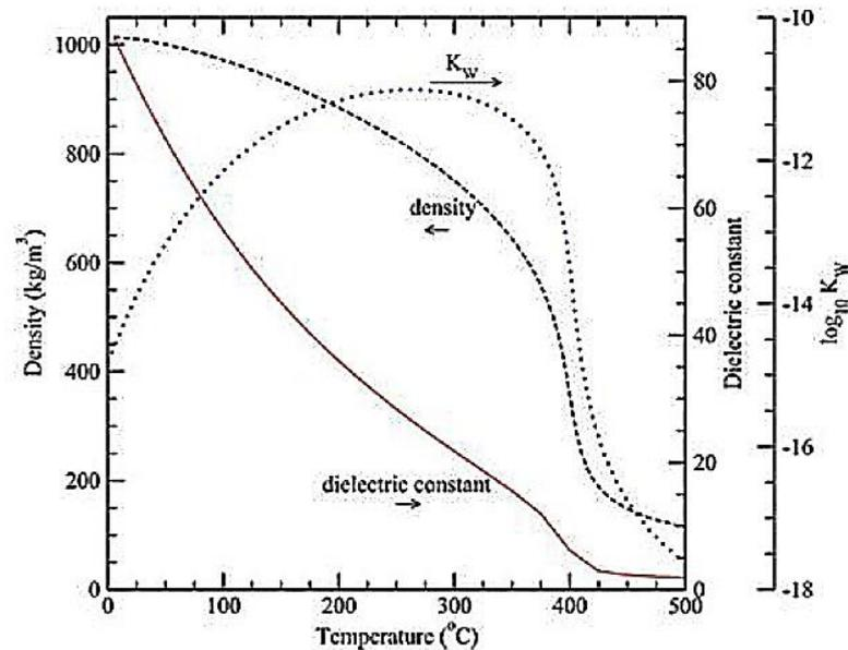
Figure 2.6 Water properties as a function of temperature at 300 bar (Johnson, 2012).
