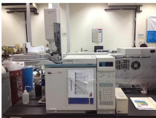
**Figure 3.7** Simulated distillation gas chromatograph (Agilent Technology 6890N).
