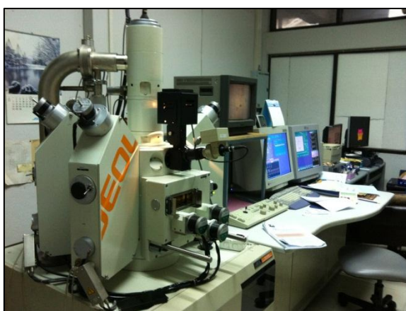
Figure 1.7 Electron Probe Micro-Analyzer (EPMA) model JEOL JXA 8100 based at Department of Geology, Chulalongkorn University.
