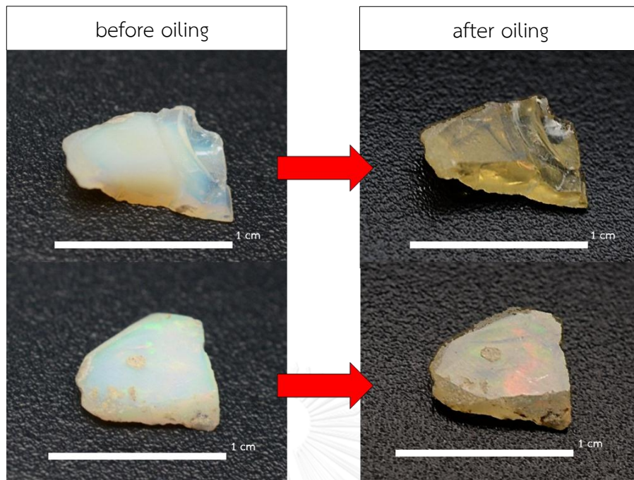
Figure 4.33 Ethiopian precious opals (samples A24 and A26) show improvement of play of color phenomena after oiling at 100°C.
