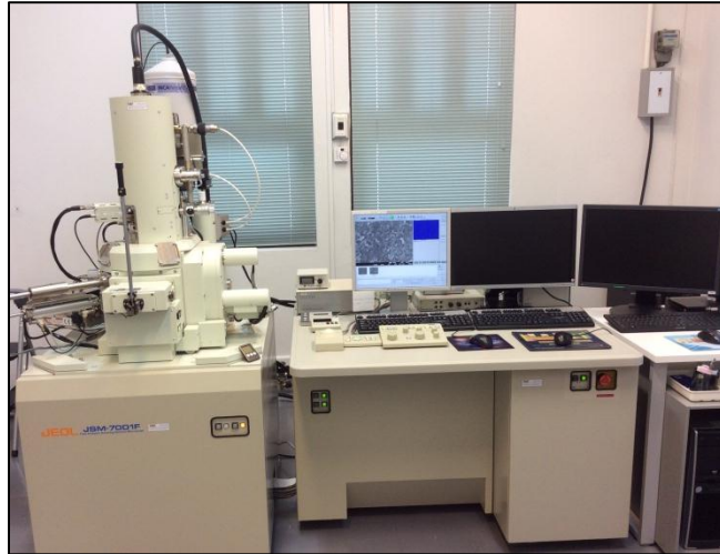
Figure 1.8 Field Emission Scanning Electron Microscope (FESEM) model JSM-7001F based at Thailand Center of Excellence in Physics (ThEP), Department of physics, Chulalongkorn University.
