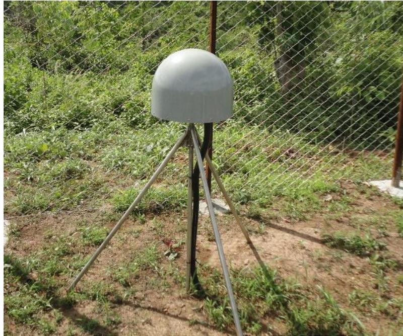
Figure 3.2 IGLE GPS station Antenna (Trimble choke ring type antenna)
