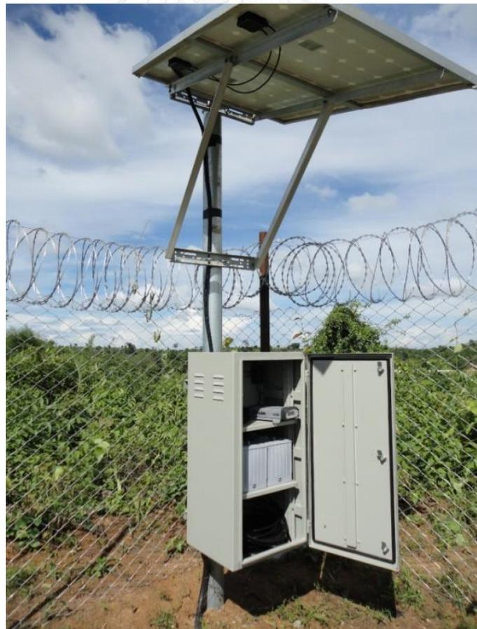
Figure 3.3 IGLE GPS station receiver box (Trimble NetR8 GNSS receiver)
