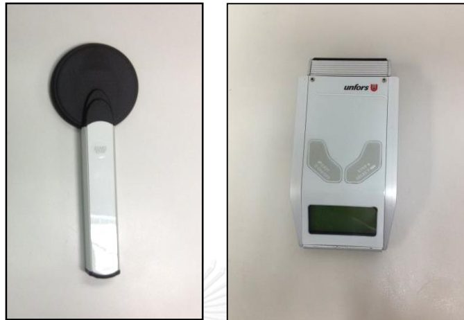
Figure 3.8: Pancake dosimeter with readout device for scattered dose received by staff.
