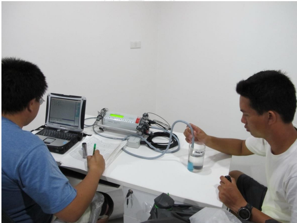
Figure 4-3. Using underwater pulse amplitude modulation fluorometer (a DIVING PAM) to measure photosynthetic efficiency of zooxanthellae.
