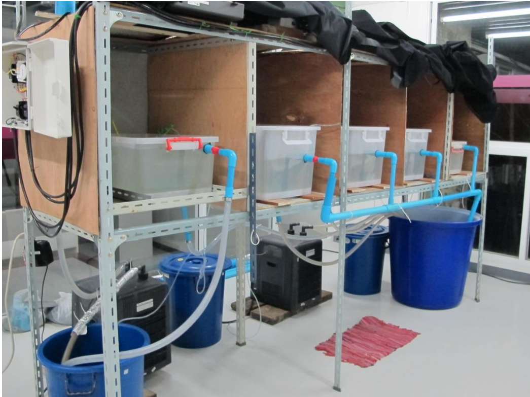
Figure 5-2. A rearing system for light intensity and photoperiod experiment.
