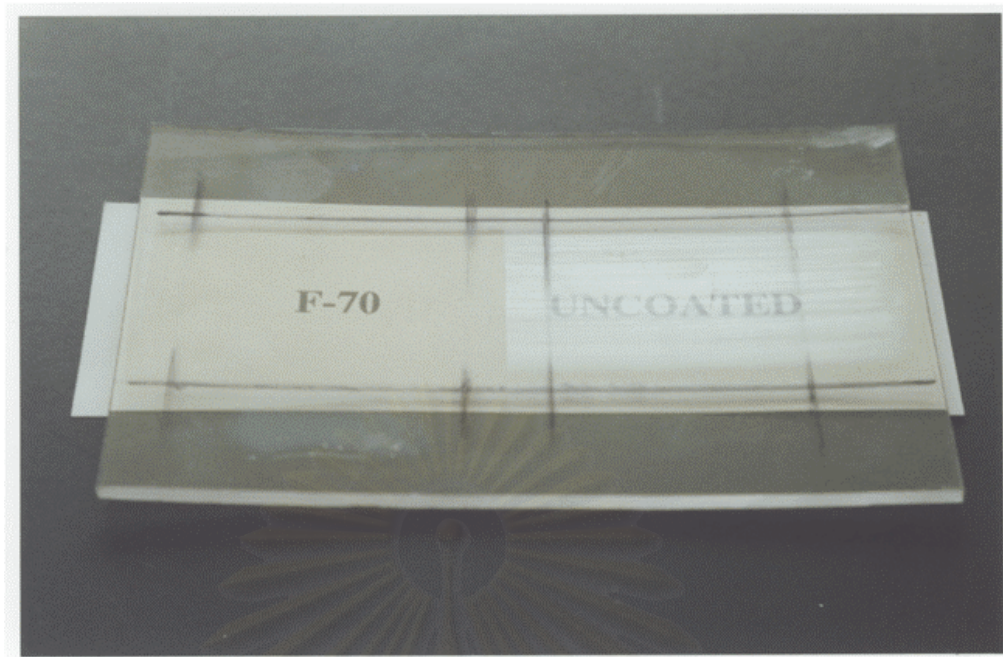
Figure 4.13 example of uncoated/coated film on the PC substrate.
