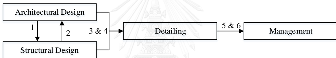
Figure 2.3: A simplified workflow of precast model exchanges (Eastman et al., 2012)
