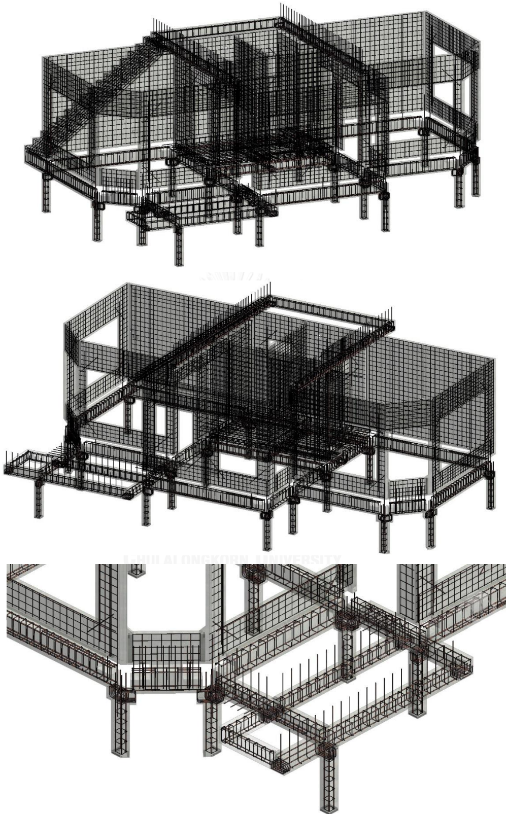
Figure B.13: Three-dimensional images of reinforcement bar
