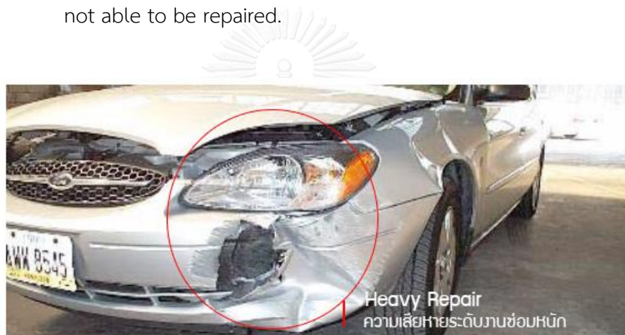
Figure 4-9 An example of heavy severity level. Reprinted from (sbrand co., ltd, n.d.)
