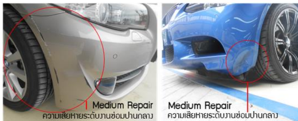
Figure 4-8 Examples of medium severity level. Reprinted from (sbrand co., ltd, n.d.)
