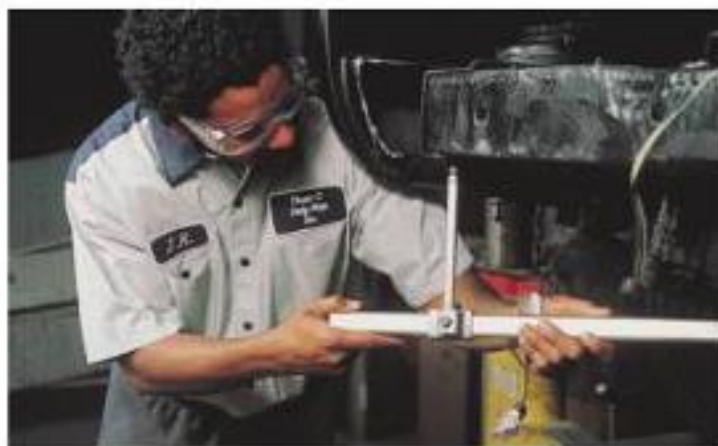
Figure 2-11 An example of tool used for measuring efficiency of body alignment. Reprinted from (Duffy, 2015)
