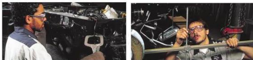
Figure 2-13 Structural panel replacement with specific tools. Reprinted from (Duffy, 2015)
