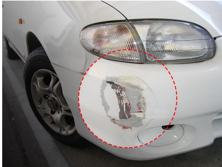
Figure 2-8 An example of minor dent damage with painting scratch. Reprinted from (honeyiscratchedthecar.com, n.d.)
