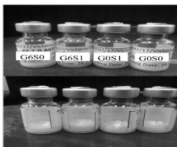
Figure 41. Physical appearances of lyophilized LAIV vaccine products of G6S0, G6S1, G0S1 and G0S0 after 28 days of storage at 30°C/75%RH
